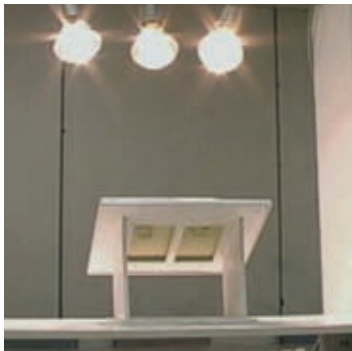
A bank of infrared lamps is arranged to shine on test materials mounted at an angle approximating a roof exposure.
